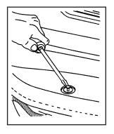
1. Remove the push pins from the air filter access panel.
